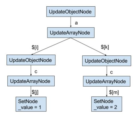
UpdateDriver::update() calls UpdateObjectNode::apply({a: [{b: 0, c: [0, 1]}]}), which calls UpdateArrayNode::apply([{b: 0, c: [0, 1]}]). This iterates through each element of the array. It finds that {"i.b": {\$gte: 0}} and {"k.b": {\$lte: 0}} both apply to the first element, so it clones and merges those children:
