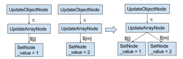
It then calls UpdateObjectNode::apply( $\{b: 0, c: [0, 1]\}$ ), which calls ArrayUpdateNode::apply([0, 1]). This iterates through each element of the array. It finds that only  $\{j: 0\}$  applies to the first element, so it calls SetNode::apply(0). It finds that only  $\{m: 1\}$  applies to the second element, so it calls SetNode::apply(1).
